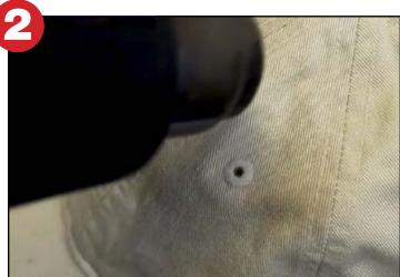
Cure the pretreat at 300°F with a Heat Gun or Dryer. When using a heat gun, keep the heat gun in motion, moving it back and forth across the pretreated area.
