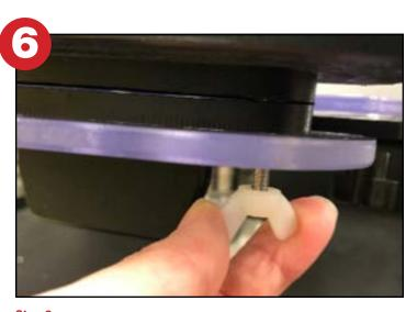
From underneath take the 2 plastic wing nuts and screw them on to the brackets screws from underneath to secure the insert to the platen.
