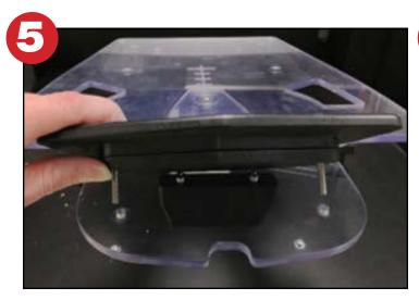
**Step 5:**With the platen in place on the printer, set the spacer if needed and then the size insert you want through the matching holes in the platen.
